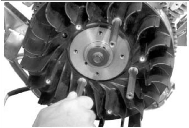
Figure 11-32. Installing Supports for Metal Grass Screen.
